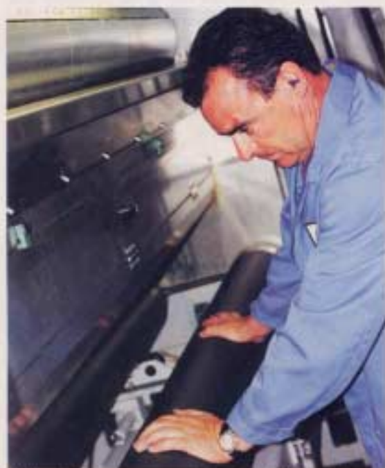
Anilox roll change is easy and automated with the Bobst Masterflex. While another job is running on the press, automatically lifted anilox rolls are positioned for immediate exchange during setup for the new job.
