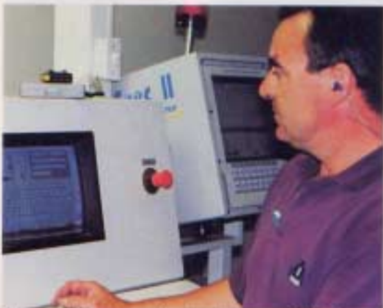
The computerized console and touch-screen of the Bobst Masterflex give total remote control. To save time, up to 5,000 specific jobs can be memorized and when one is reprinted, the press automatically re-configures.
